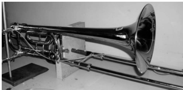
FIG. 1. Picture showing some details of the experimental setup used for sound pressure pulse measurements in a slide trombone.
